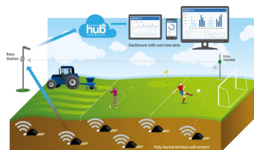
Figure 1: Wireless Soil Moisture Sensors [24]
